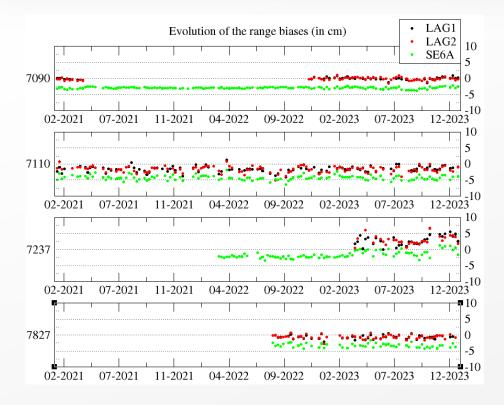
For Sentinel-6, a range bias is estimated for every station if measurements are available, whereas for the spherical satellites, a bias is estimated only if it's not to be found in the DHF for the given period.
