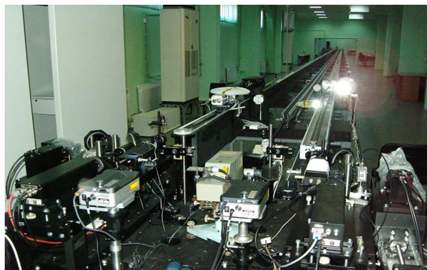
Fig.5. The Special Standard of Length to 60 m
