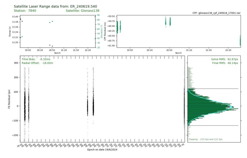
This variation in RMS is due to the angle at which the retro-reflector array is observed.
