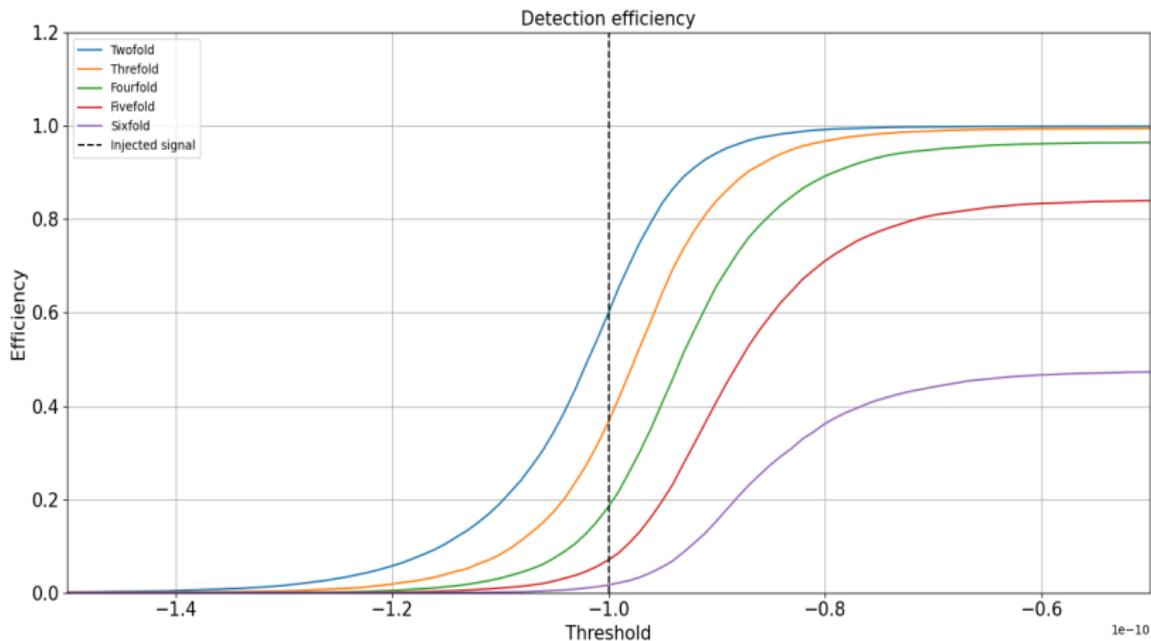
**Figure:** Detection efficiency curves for  $k \sim 10^4$  events with  $A \sim -10^{-10}$  s. As the number of clocks becomes 6, the probability that a DW hits the ground clock and a satellite one (within 30 s) gets larger and the sixfold is missing.
