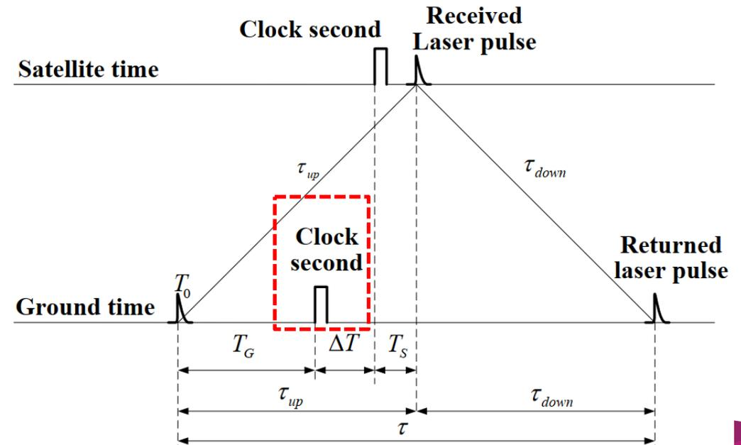
$$R = c * (t_{receive} - t_{send} + \Delta t) / 2 + \varepsilon$$
