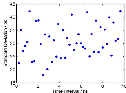
High precision time comparison based on GNSS PPP, real-time time synchronization is less than 0.2ns
