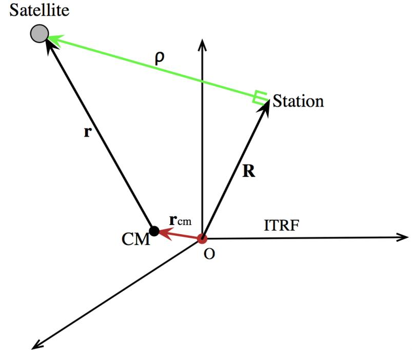
Geocenter motion and gravitational spherical harmonic coefficients are estimated during POD process, together with some other parameters used to absorb errors
